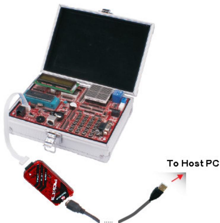
Figure 6 – PICkit3 ND118-4520 Connection Diagram
