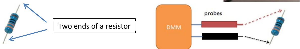
Fig. 12 (a) A resistor (b) Measuring a resistor with DMM
