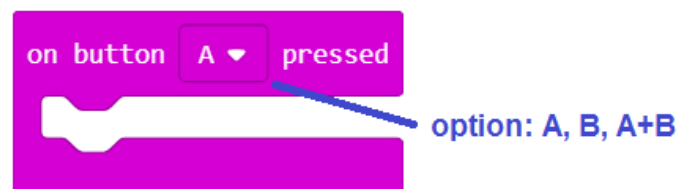
Fig.5 Button event function block
