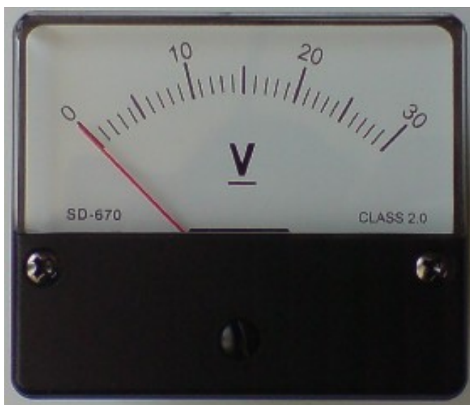
Fig 17: Image of typical voltage with a measuring range up to 30V .
